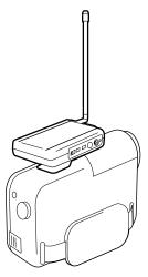
PRO 88W receiver mounted to video camcorder accessory shoe or supplied Velcro tape
